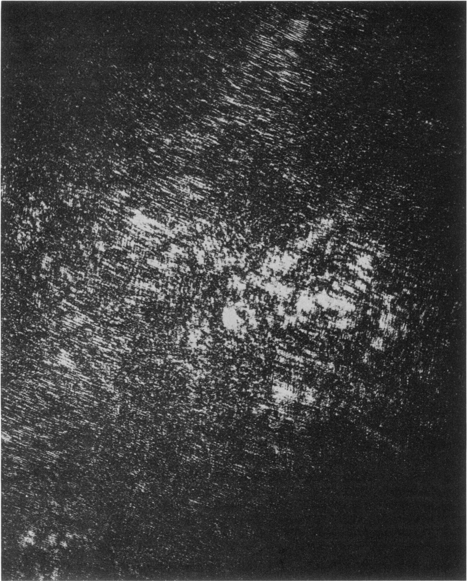
FIGURE 1 Fringe pattern as observed in a plane 10 cm from the swimbladder with the laser pencil focused onto the swimbladder and passed through both walls of the preparation. The photograph was taken without a lens and the Panatomic X film was exposed for approximately 1 s. The enlargement was made so that the optical axis is close to the center of the figure. The maximum angle of scattering shown in the enlargement is approximately 5^\circ . The preparation was optically more dense than was normally used in our experiments. Blurring of some of the fringe patterns is a result of the natural fluctuations of the medium.
